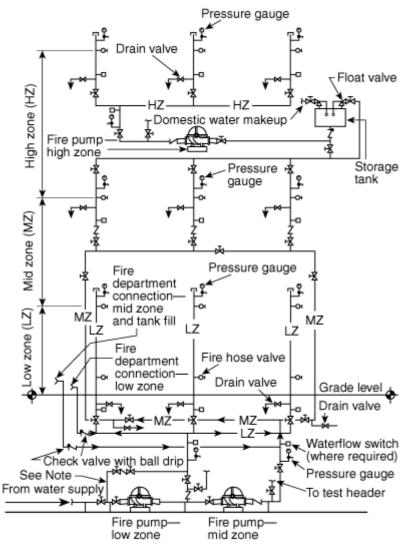
Note: Bypass in accordance with NFPA 20, Standard for the Installation of Stationary Pumps for Fire Protection.
